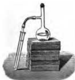
FIG. 1.—Evolving a gas by use of a side-neck flask.
