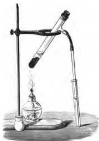
FIG. 2.—Evolving a gas by use of a side-neck test-tube.
