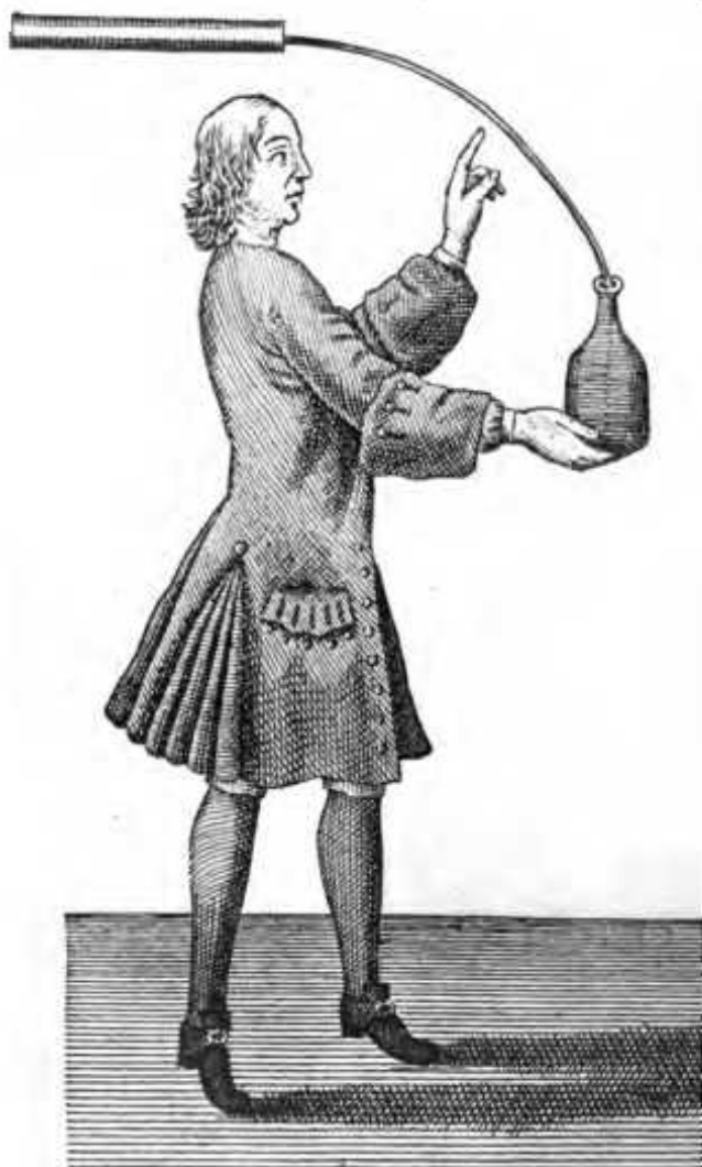
The Leyden experiment. The first storage of electricity
