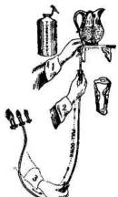
The Syphon Syringe has but one piece of rubber tubing eight feet long, a metal U-shaped holder at the summit, a sinker on the inlet end, a combined syphon starter and shut off. The combined starter and shut off is perfect for either starting or stopping the flow.
