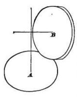
angles with each other, then it will be evident, from mere inspection, that when B has turned once on its axis it will have gone once around A. Thus B will have gone once around the axis of A, and once about its own axis. Next, incline the axis of B upward, so as to approach a parallelism to A, and the same result will be seen from mere inspection,
