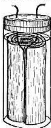
FIG. 1. — Original type of Planté accumulator. (About \frac{1}{2} full size.)
