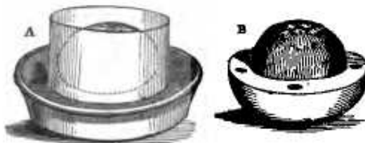
The cut above shows the moulding of the orange; A, represents it half buried in the sand, with the tin or paper around; B, is a view of the first half mould when complete.
