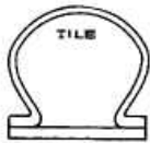
Pallet End view of Horse Shoe Tile, the first drain tile made.
