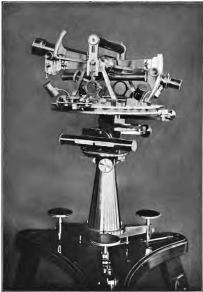
Old 10-inch Theodolite of Everest design, used on the early Indian Survey.
