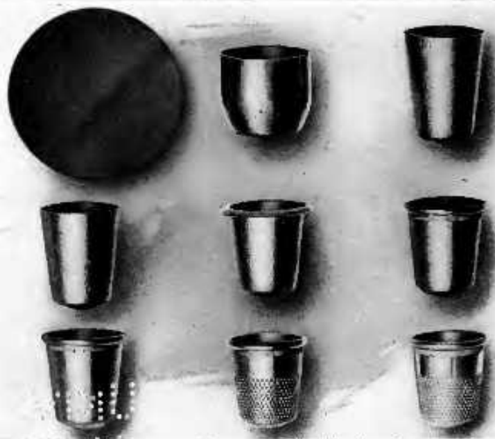
Courtesy of Scoville Manufacturing Company Sailmaker's Thimble Stages in the Manufacture of a Thimble
