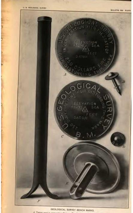
A. Tablet used in cooperating States. The State name is inserted at G. B and D. Cooper temporary bench mark, consisting of a nail and copper washer.  $A_i$  C, and A. Tablets for stone or concrete structures. F. Iron part used where there is no rock.
