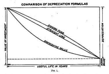
It should be observed that none of these formulas takes into consideration interest on investment, output, cost of operation, or maintenance charges. Figure 1 gives a graphic comparison of the above formulas.
