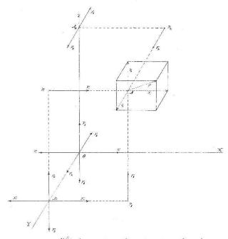
This is most readily done by reflering all the forces to three coordinate ares at right angles to each other with origin at the most convenient point. Let 0x, 0x + 0x be these axes, I let the forces in the directions of X, X > Z from 0 be considered
